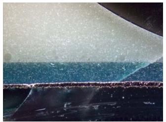
**Figure 1.** Crack in fillet of underfill encapsulant propagates into board.
